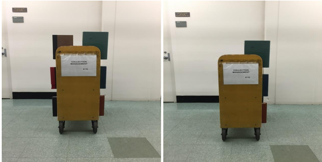
DO DON'T Figure 2. –Loading books onto only one side of a book truck may cause it to tip over.
